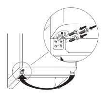
Open the freezer compartment door and fit the plinth.
